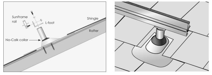
Cut an opening in the roofing material over a rafter to accommodate the flashing riser. Install the standoff, ensuring that both lag bolts are screwed into the rafter. Insert the flashing under the shingle above and over the shaft of the standoff. No-Calk collar does not require sealing of the flashing and standoff shaft.
