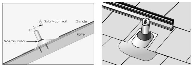
Cut an opening in the roofing material over a rafter to accommodate the flashing riser. Install the standoff, ensuring that (1) both lag bolts are screwed into the rafter, and (2) the raised flange is oriented parallel to the rail. Insert the flashing under the shingle above and over the shaft of the standoff. No-Calk™ collar does not require sealing of the flashing and standoff shaft.
